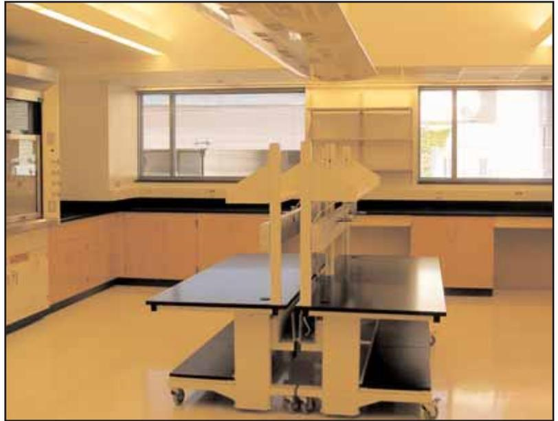
**The research labs are open labs with no "anchor" type functions which would impede their flexibility. Overhead service carriers with all utilities greatly contribute to the flexibility.**
