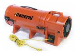
lighter, more economical alternative to steel units. The EP8ACP15 is ideal for supplying fresh air to confined spaces in nonhazardous locations. It can also be used for a variety of other tasks, such as drying damp areas and cooling personnel in utility trenches. The EP8ACP15 offers an 8-inch output diameter and produces 900 CFM of free air flow. It is powered by a singlespeed, one-quarter-horsepower motor, which operates from a standard 115volt electrical outlet. To learn more
