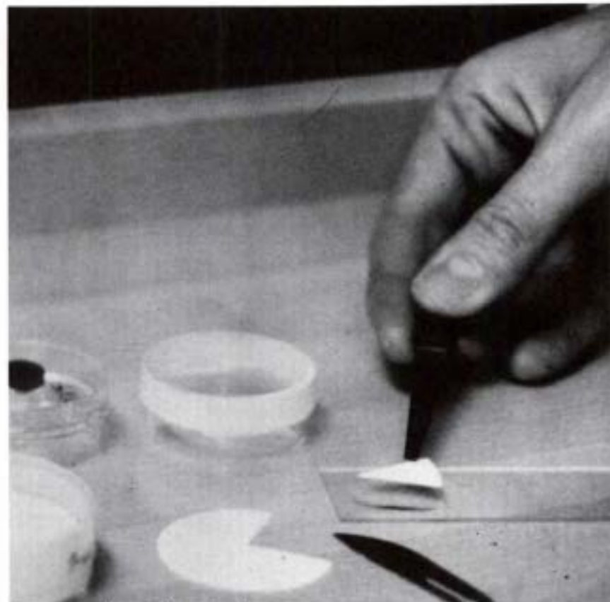
Mounting asbestos filters for phase contrast microscopy.
