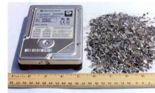
After passing through a disintegrator, computer hard drives end up as tiny bits of "e-scrap."
