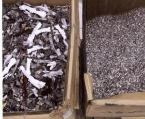
Computer parts and other metal waste end up as "e-scrap," some of which can be recycled. Powerful shredders reduce metal to strips (left) that can be run through a disintegrator and pulverized to tiny bits (right) for added security.
