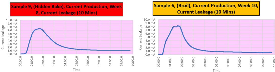
The leakage current is back within acceptable limits within 4 to 5 minutes and will stay there when in operation after this initial startup. The range safety standard does not currently measure leakage current above 125 Volts(see clause 55).
