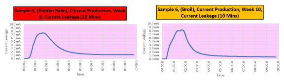
The leakage current is back within acceptable limits within 4 to 5 minutes and will stay there when in operation after this initial startup. The range safety standard does not currently measure leakage current above 125 Volts(see clause 55).
